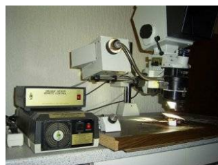
Stereo Dynascope for visual inspection
