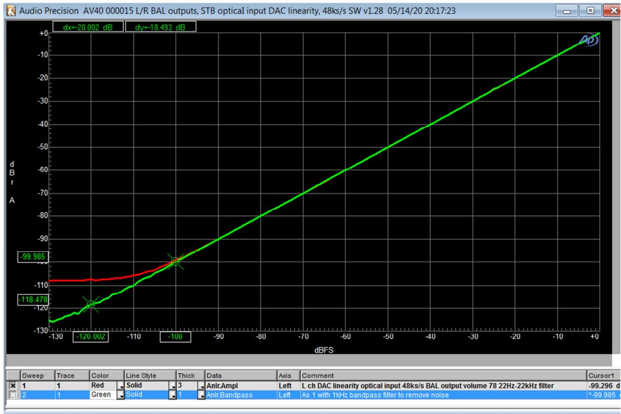
The red curve was with a 22Hz-22kHz filter in the analyser; below about -105dBFS input internally generated white noise in the AV40 started to intrude on the output.
