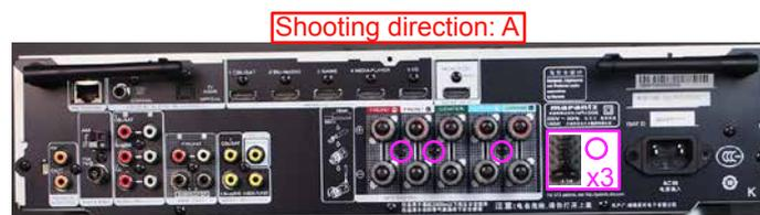
(2) Remove the screws. Remove the CORD HOLDERS and connector wires.
