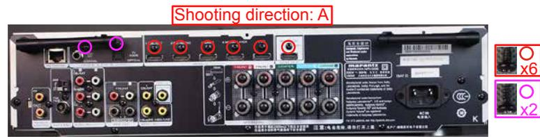
(2) Remove the CORD HOLDERS. Cut the wire clamp, then remove the connector. Remove the FFC.
