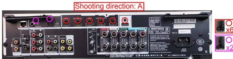
(2) Remove the connector PCB.
