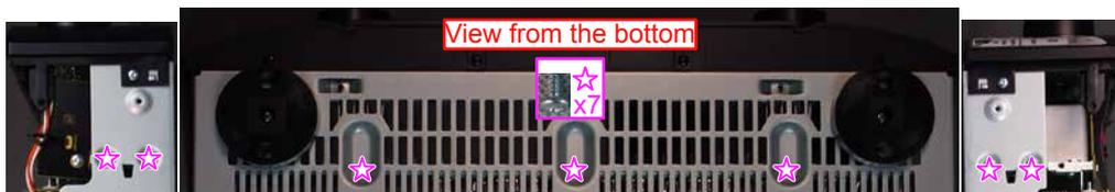
(2) Remove the screws. Cut the wire clamp, then remove the connector. Remove the FFC.
