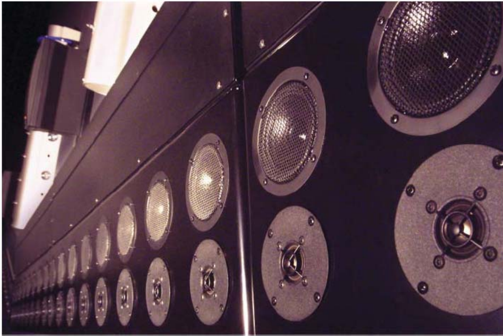
Figure 9-8: Loudspeaker panels equipped with eight two way speakers and eight amplifiers each.
