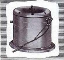
TYPE V 1000 — This vibrator is designed to produce a peak alternating thrust of ±500 lbs. (unblown) at 1 kW. A forced draught into the vents provided in the base will allow increased input current for a correspondingly increased thrust. Unit construction has been adopted and careful attention to detail has produced a vibrator that can quickly and easily be stripped and reassembled should repairs become necessary—the design is such that no routine maintenance is required.
