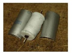
FT3 uses aluminum casing and thin tabs as leadouts while K72 uses thicker steel casing with solid poles as leadouts. FT3 is glass-encapsulated while K72 is hermetically sealed, and due to the thick steel case, K72 is even heavier than FT3.
